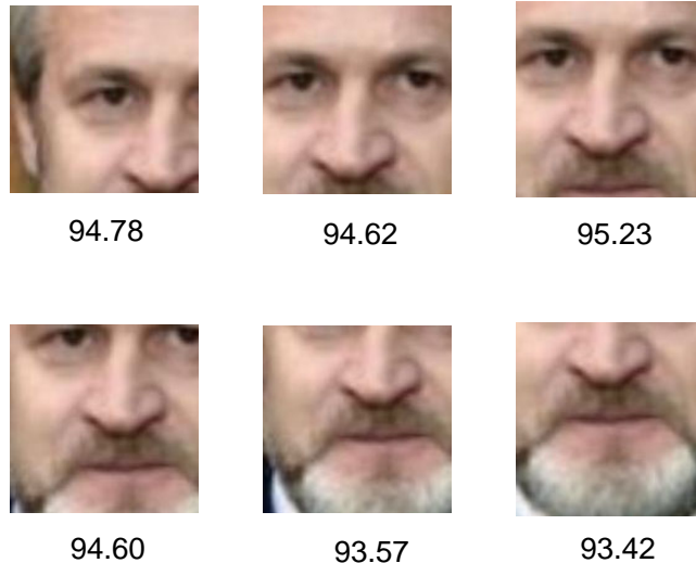
Figure 4: The verification accuracy (%) of an individual patch on LFW. The features are extracted from the model CNN-1 constructed on the basis of ResNet.
